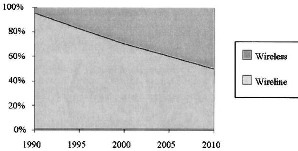
FIG. 2. Growth in wireless vs. wireline. (Source: MITRE Corporation.)
