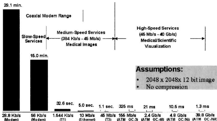
FIG. 4. Image transmission times.
